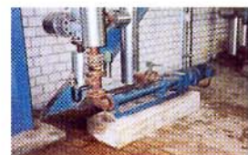
Crystallization VFD controlled seepex pump BN 5-12, product: molasses, flow: 1.7-5 m 3 /h / 7.5-22 usgpm, speed: 165-400 rpm, pressure: 6.72 bar / 96 psig, temperature: 55° C / 131° F, viscosity: 7000 mPas, SG: 1.4 kg/dm 3
